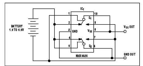
This circuit senses battery polarity and then quickly connects the load or swaps the battery leads.
